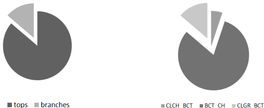
Figure 8. Base case logistics optimized. Tops were the primary biomass extracted with top material typically moved with a self-loading log truck directly from the landing and sent to the BCT for processing and conversion. A small portion of branches were sent to centralized yards for processing before delivery to the BCT for conversion.
