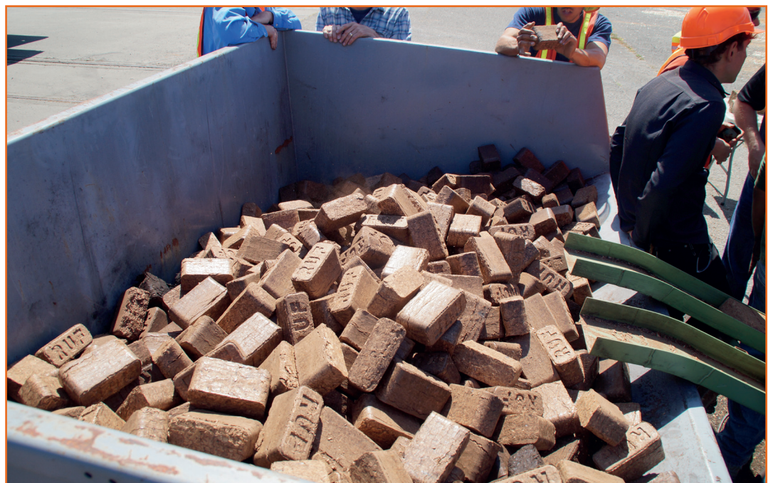
Final torrefied briquettes from Biogreen CM600 torrefier in W2W project. July 2016, Arcata, CA
