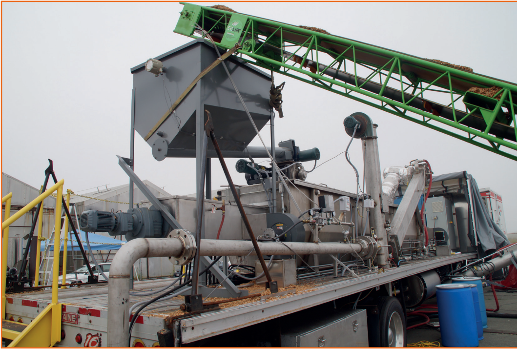
Biogreen model CM600 torrefaction system. Reactor sitting on a mobile trailer during testing for W2W project in July 2016, Arcata, CA
