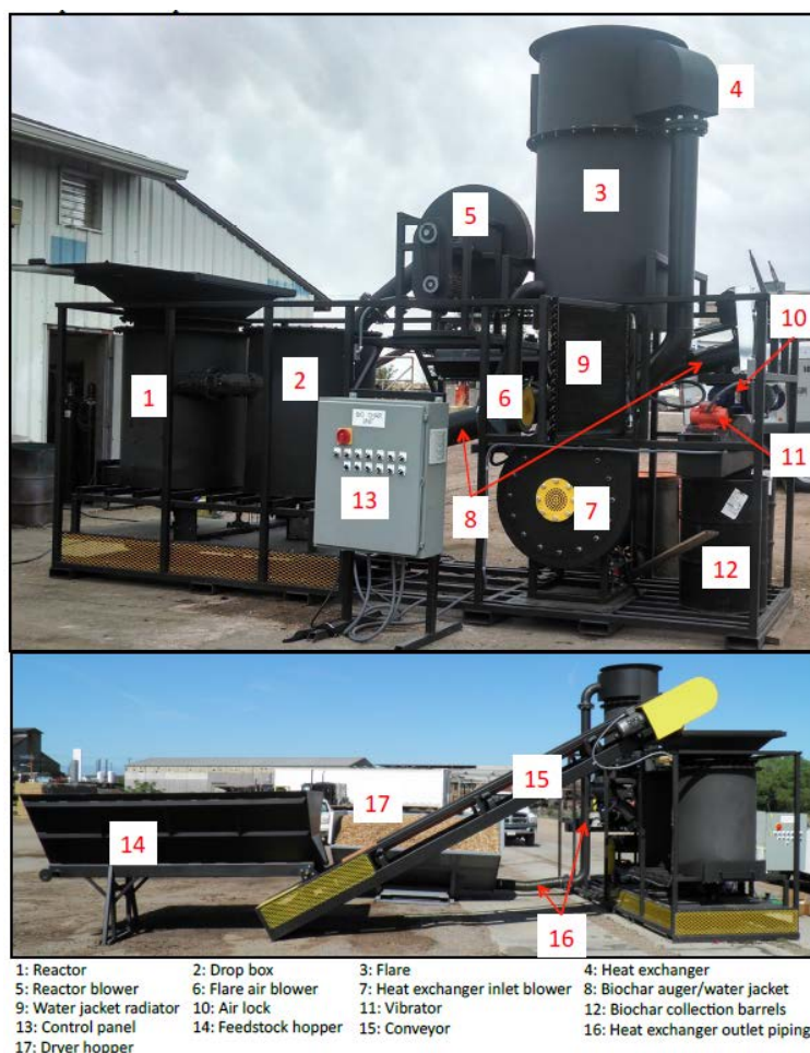
Figure 3 BSI biochar production system. Image credit: Schatz Energy Research Center.
