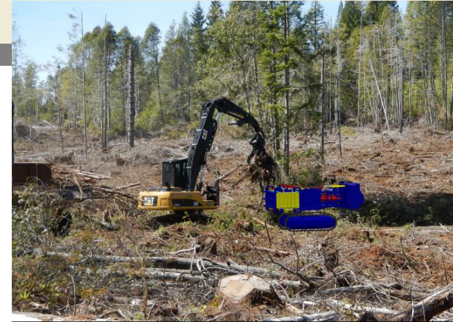
Conceptual tracked baler drawing on actual biomass recovery operation at Arcata, Calif. Current bulk biomass forwarder shown to left of loader.
